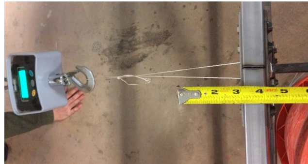
Figure 19: Lateral Load Test Photo By: Isaac Block
