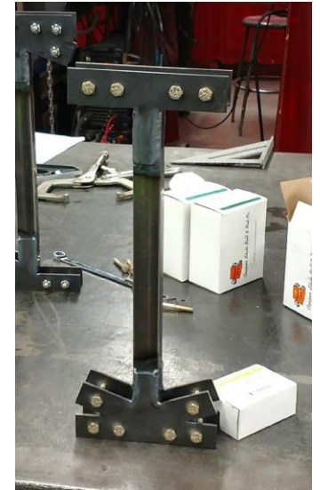
Figure 10: Fabricated Vertical Truss Member with Welded Plates Photo by: Matthew Parrish
